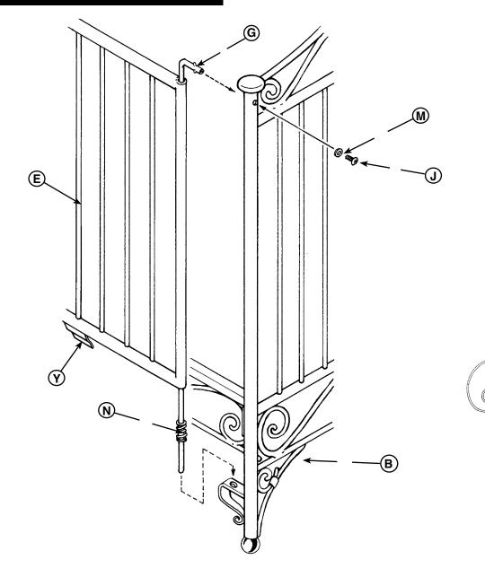
Slide one of the slide rods (G) through either of the thin tubes of the front gate, making sure that the latch brackets (marked with a Y) are on the bottom inside. Place a spring (N) onto the end of the slide rod, and insert the end into the bottom bracket. Insert the top end of the slide rod into the top hole of the side piece and fasten it using one of the large short machine screws (J) and large star washer (M). Now repeat the process on the other side.
