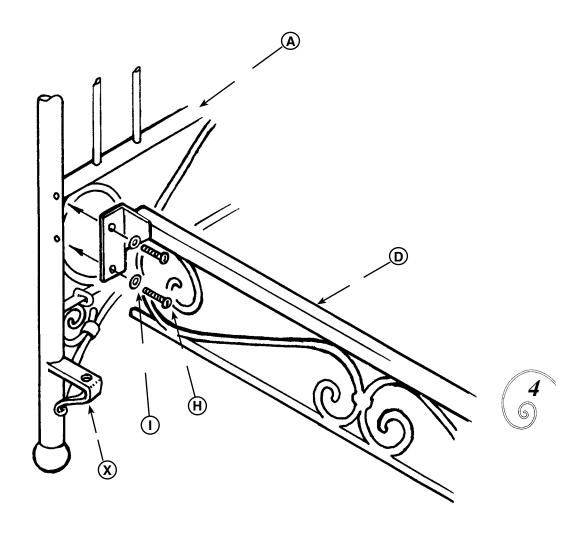
Attach the front brace (D) to the front of the crib using the small machine screws round head (H) and the 4 small star washers (I). Tighten machine screws with a screwdriver.
