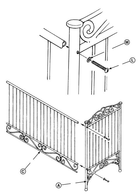
Using a screw driver, attach back piece (C) to side pieces (A) and (B)(not shown) as indicated using 4 large machine screws (L) and the large star washers (M). Make sure that the brackets on the bottom of the side pieces (see figure 2 marked (X)) are pointing inside the crib. Make sure that the screws are snug.
