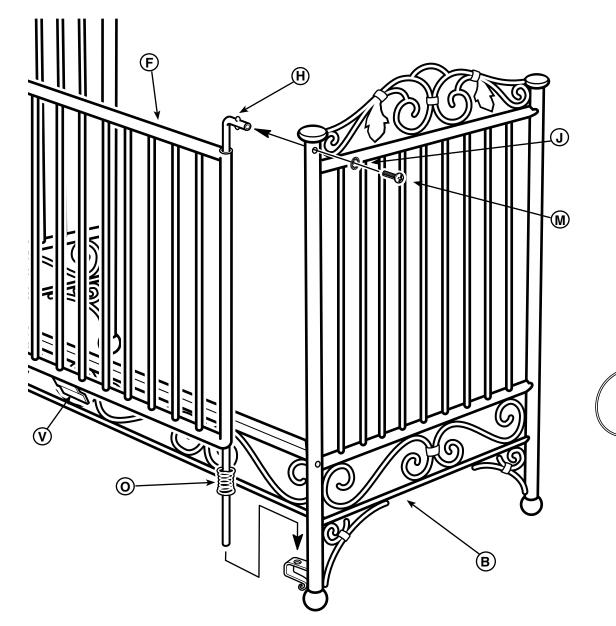
Install the front gate (F) one side at a time as shown. Be sure to place the spring (O) onto the bottom of the slide rod (H) before inserting it into the bottom bracket of the crib. Insert the top end of the slide rod into the top hole of the side piece and fasten it using one of the large short machine screws (M) and large star washer (J). Now repeat the process on the other side.
