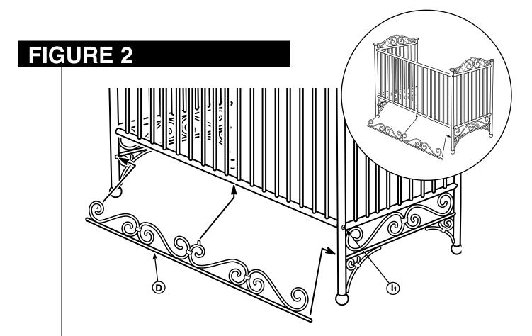
Install the back scroll detail (D) by simply slipping in the 3 points as shown. Now tighten the machine screw ( $I_1$ ) from figure 1.
