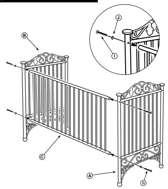
Using a screw driver, attach back piece (C) to side pieces (A) and (B) as indicated using 4 large machine screws (I) and the large star washers (J). Make sure that the brackets on the bottom of the side pieces (see figure 3 marked (X)) are pointing inside the crib. Leave the bottom machine screw (shown as I<sub>1</sub>) loose (about 1/2"). Make sure that the remaining 3 screws are snug.
