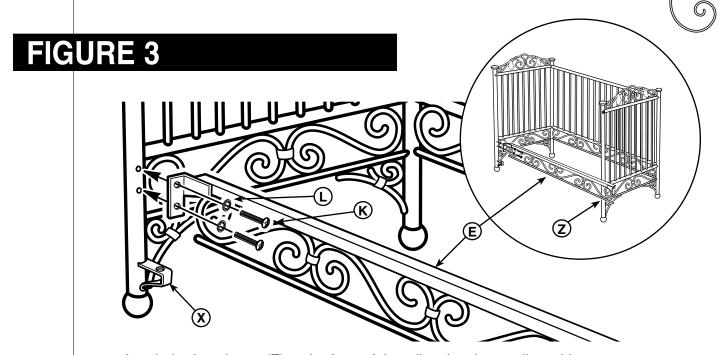
Attach the front brace (E) to the front of the crib using the small machine screws (K) and the 4 small star washers (L). Once installed, make sure that the bottom section of the front brace can swing back freely. If it cannot, make sure that the brace is behind the stop in the area shown as (Z). Tighten machine screws with a screwdriver.
