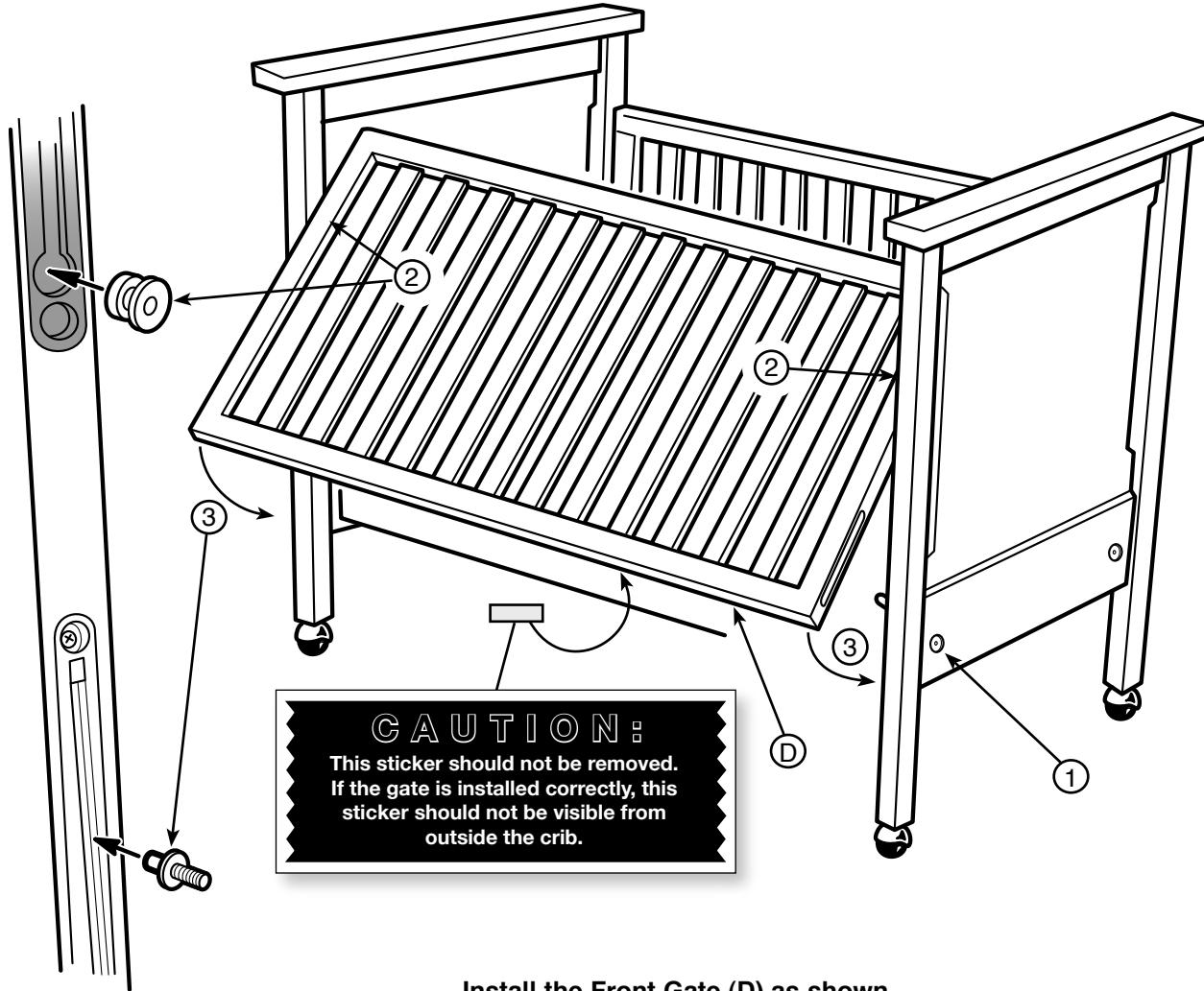
**Install the Front Gate (D) as shown.**
