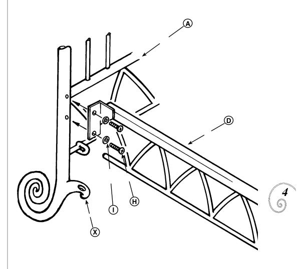
Attach the front brace (D) to the front of the crib using the small machine screws round head (H) and the 4 small star washers (I). Tighten machine screws with a screwdriver.
