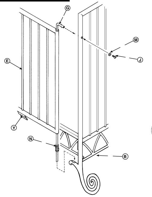
Slide one of the slide rods (G) through either of the thin tubes of the front gate, making sure that the latch brackets (marked with a Y) are on the bottom inside. Place a spring (N) onto the end of the slide rod, and insert the end into the bottom bracket. Insert the top end of the slide rod into the top hole of the side piece and fasten it using one of the large short machine screws (J) and large star washer (M). Now repeat the process on the other side.
