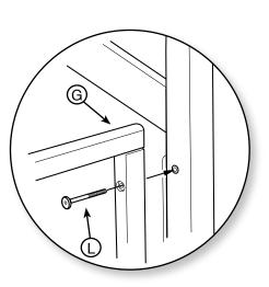
Attach the Back Piece (G) using the 4 remaining Long Machine Screws (L). Use the Hex Tool (T) to tighten these screws. Now tighten the 4 Long Machine Screws shown as (L<sub>1</sub>) using the Hex Tool.
