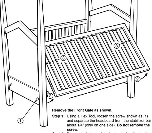
**Step 2:** Detach the bottom of the front gate by slipping the metal guide pin out of the plastic track on both sides.
