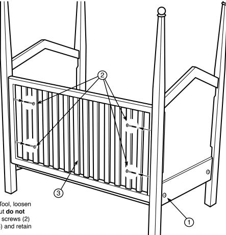
Turn the crib around. Using the Hex Tool, loosen the screw (1) on the side of the crib but **do not remove the screw**. Now remove the screws (2) as shown. Remove the back piece (3) and retain all parts for future use.
