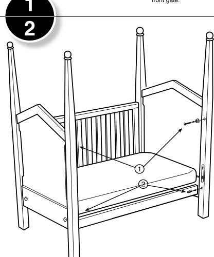
Remove the plastic bushings (1) and the metal guide pins (2) using a Phillips head screwdriver. Keep the parts in a safe place, as you will need them if you wish to use it as a crib again.
