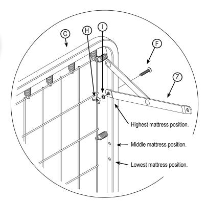
Position the Mattress Support Legs (Z) as shown (follow the guide below for the correct height for your child) and install the Medium Machine Screw (F), Star Washer (I) and the Wing Nut (H). Tighten by hand. Repeat on the remaining 3 Legs.
