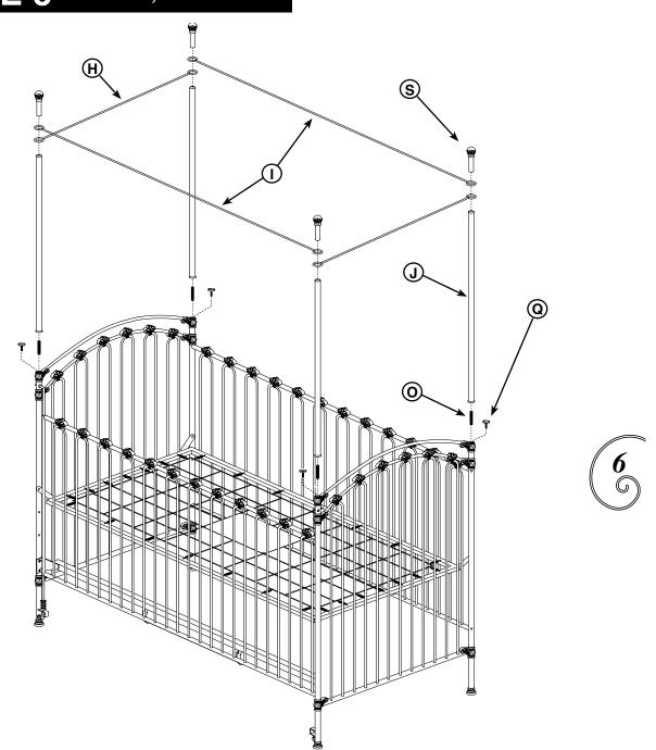
**A. Low crib setup:** If you choose not to set up this crib as a 4 poster, or canopy, attach the threaded disc covers (Q) to the top of the corner posts. Tighten (Q) by hand. Assembly is now complete.
