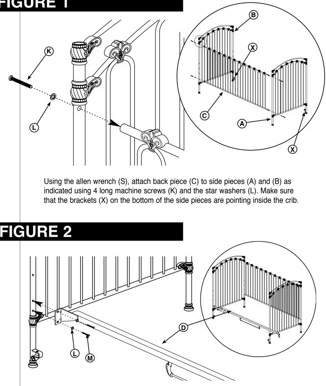
Using the allen wrench (S), attach the stabilizer/latch bar (D) to the front of the crib using the medium machine screws (M) and 4 star washers (L).
