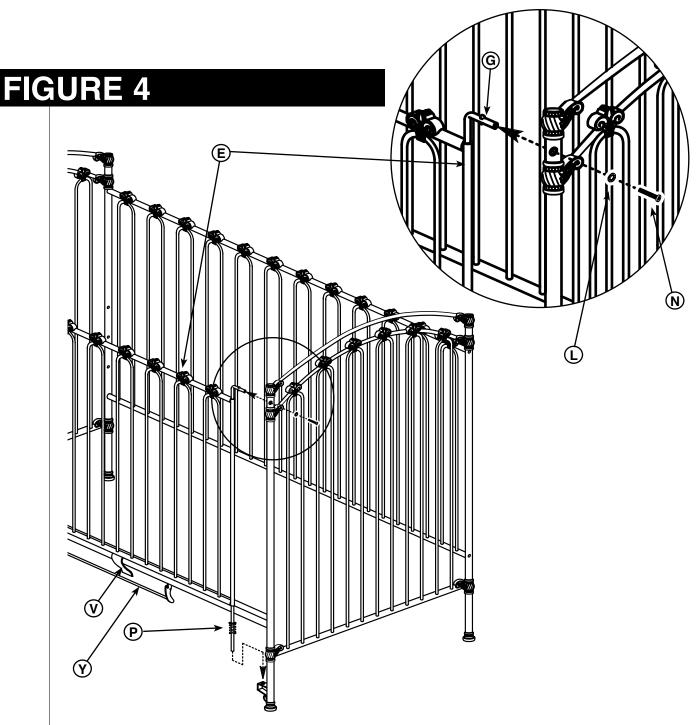
Install the front gate (E) as shown, latch plate (V) pointing inside. Insert the slide rods (G) through the tubes on the gate, and place the springs (P) onto the bottom of the slide rods before inserting it into the bottom brackets of the crib. Insert the top ends of the slide rod into the top holes of the side pieces and attach them using the short machine screws (N) and star washers (L).
