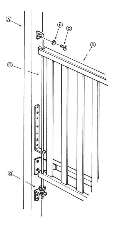
Finaly, install the Front Gate with the strike plates pointing inside the crib. Insert one of the Slide Rods (G) throught he top hole of the gate, then through the top bracket, then through the hole on the bottom of the Front Gate, through one Spring (Q) and finaly through the L Bracket. Attach the slide rod using 1 Short Machine Screw (O) and 1 Split Washer (P). Now repeat on the other side.
