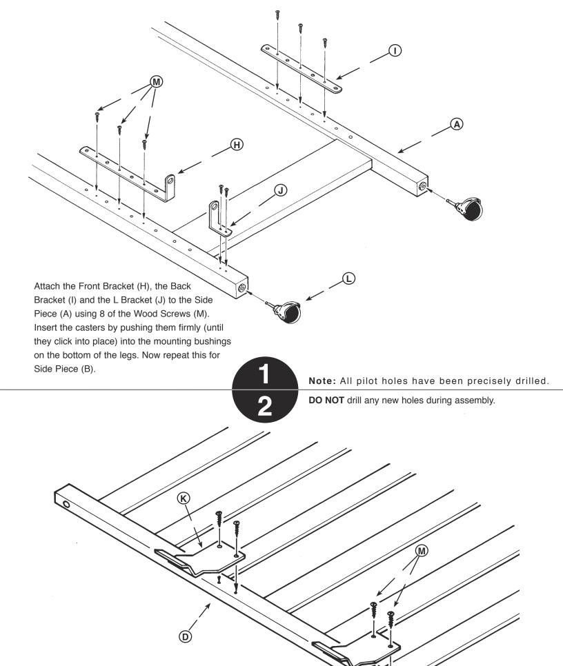
Attach the 2 Strike Plates (K) to the front gate using 4 of the Wood Screws (M). Note, the
