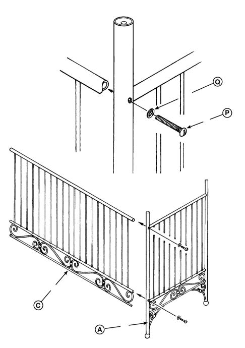
Using a screw driver, attach back piece (C) to side pieces (A) and (B)(not shown) as indicated using 4 large machine screws (P) and the large star washers (Q). Make sure that the brackets on the bottom of the side pieces (see figure 2 marked (X)) are pointing inside the crib. Make sure that the screws are snug.
