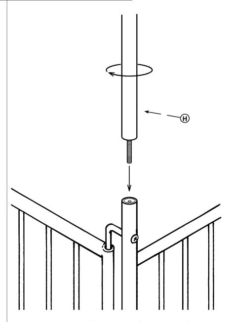
Attach Corner Post Extensions (H) by screwing each of them into the top of the two side pieces (A & B). Please make sure that the poles are tightened firmly by hand.
