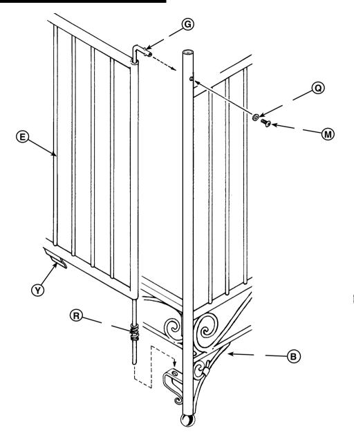
Slide one of the slide rods (G) through either of the thin tubes of the front gate, making sure that the latch brackets (marked with a Y) are on the bottom inside. Place a spring (R) onto the end of the slide rod, and insert the end into the bottom bracket. Insert the top end of the slide rod into the top hole of the side piece and fasten it using one of the large short machine screws (M) and large star washer (Q). Now repeat the process on the other side.
