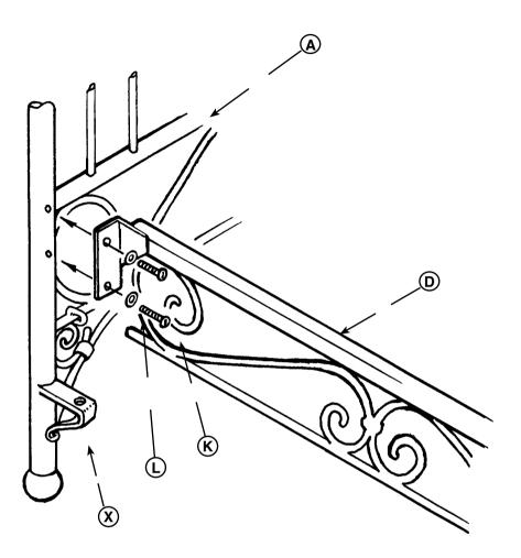
Attach the front brace (D) to the front of the crib using the small machine screws round head (K) and the 4 small star washers (L). Tighten machine screws with a screwdriver.
