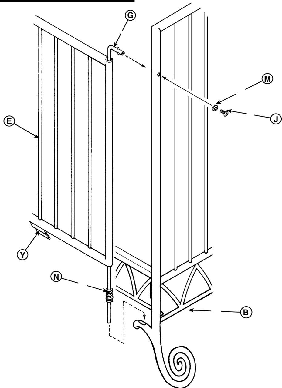
Slide one of the slide rods (G) through either of the thin tubes of the front gate, making sure that the latch brackets (marked with a Y) are on the bottom inside. Place a spring (N) onto the end of the slide rod, and insert the end into the bottom bracket. Insert the top end of the slide rod into the top hole of the side piece and fasten it using one of the large short machine screws (J) and large star washer (M). Now repeat the process on the other side.
