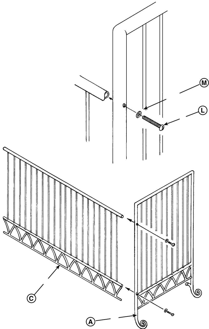
Using a screw driver, attach back piece (C) to side pieces (A) and (B)(not shown) as indicated using 4 large machine screws (L) and the large star washers (M). Make sure that the brackets on the bottom of the side pieces (see figure 2 marked (X)) are pointing inside the crib. Make sure that the screws are snug.
